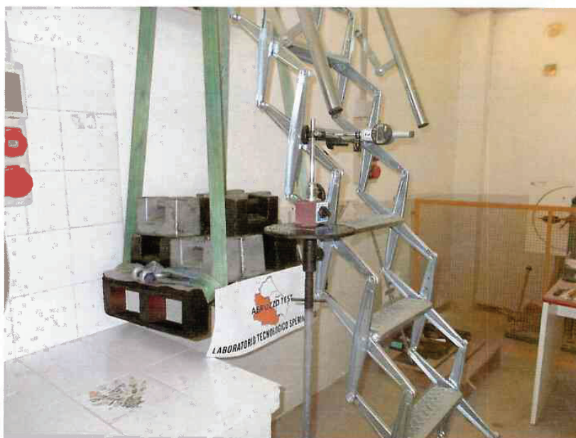
Picture 3: static load test – middle step of the ramp, specific dial gauge
