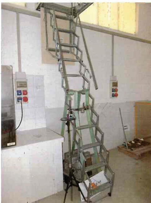
Picture 2: static load test – middle step of the ramp
