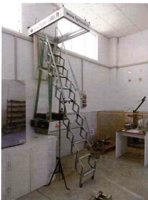
Picture 1: static load test – first step
